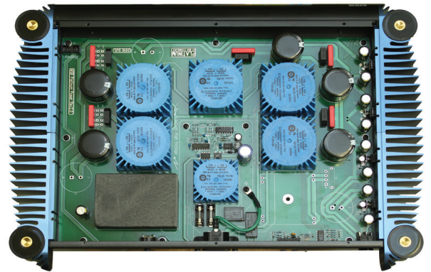
Platinum Power Base with 6 transformers.
