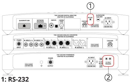
The Digital Director features an RS-232 control port on the back of the unit that can be used with whole home control systems and for home theater integration. A full list of commands and coding can be found using the OB code below.
