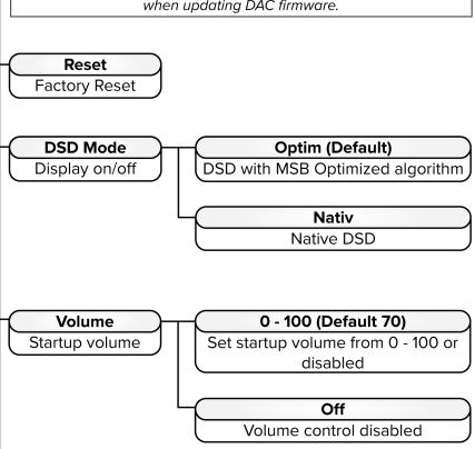
**Note:** If you choose to use the DAC with an external preamp, we recommend turning the volume control off. To do this, turn the knob past 100 to "off". If the volume is set to "off" the display setting above will also default to off since volume is no longer being used.
