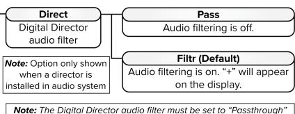
**Note:** The Digital Director audio filter must be set to "Passthrough" when updating DAC firmware.
