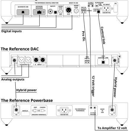
When installed properly, your system should look like the example above. The digital inputs installed in your digital director may vary depending on what sources are in your system, However; the only modules that should be installed in the DAC will be the provided Pro ISL and Control Link modules as well as any analog input modules you may have in your system.
