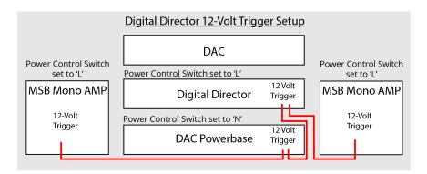
The diagram above is only a visual example and the actual connections may vary in your system. The specific order in which the units are connected does not affect how the 12 volt connections will function. The only requirements are that each unit is connected to a 12 volt trigger port of another unit in the chain. Only one unit is set to the normal 'N' position while all other units are set to the linked 'L' position.
