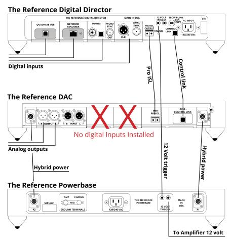
When installed properly, your system should look like the example above. The digital inputs installed in your digital director may vary depending on what sources are in your system, However; the only modules that should be installed in the DAC will be the provided Pro ISL and Control Link modules as well as any analog input modules you may have in your system.
